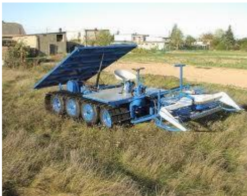
Figure 3.3 A Polish Reeda reed harvester with a BCS cutter mounted on it (Reeda Reed 2013)
