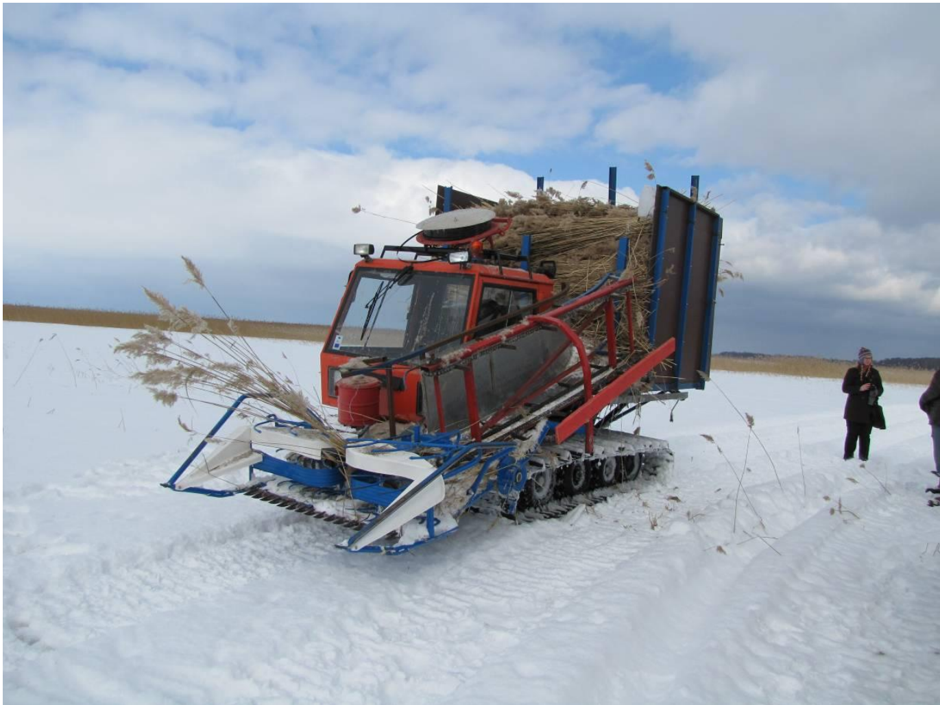
Figure 3.2 A reed harvester belonging to OÜ Järveroog with a BCS header mounted on a Paana track-tractor (Photo: K. Akermann)
