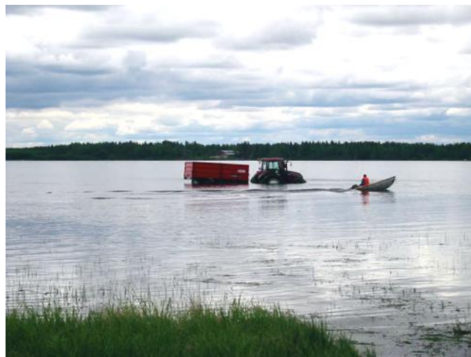
Figure 5.10 Specially equipped Valtra C150 with a trailer in tow can mow reed in the lake ( http://www.valtra.com/news/405.asp )
