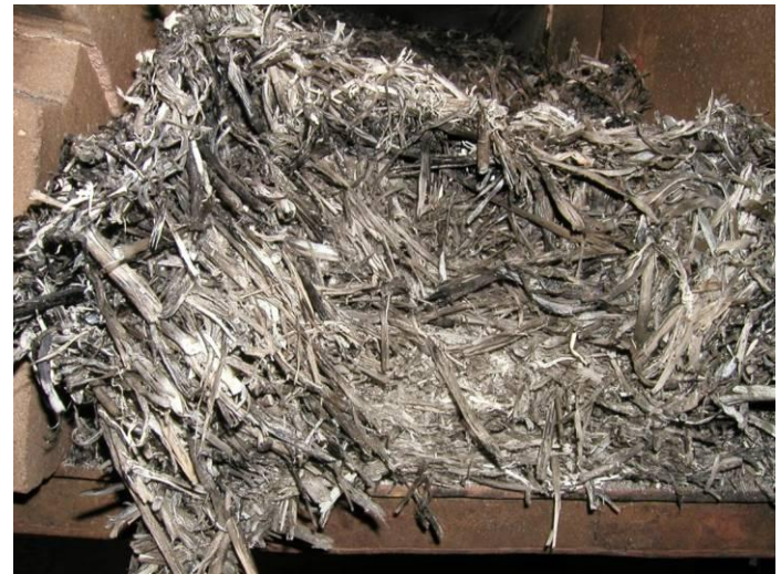
Figure 4.12 Reed ash residue after the combustion test (Photo: Ü. Kask)
