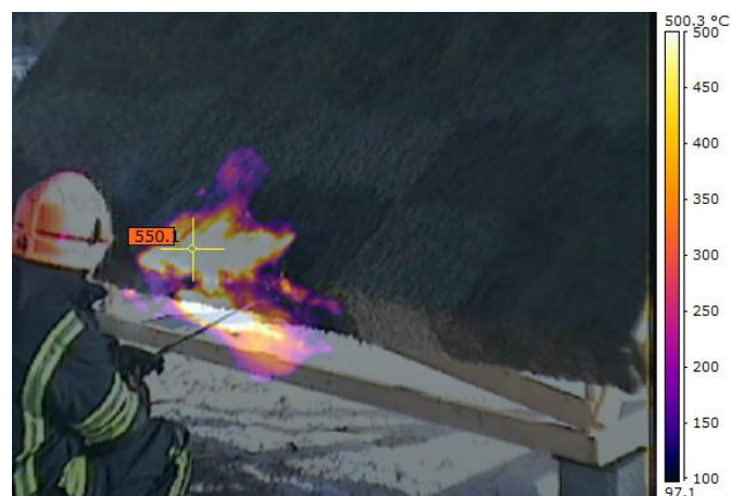
Figure 3.36 A thermal picture of the roof No 1. The lighting is going on
