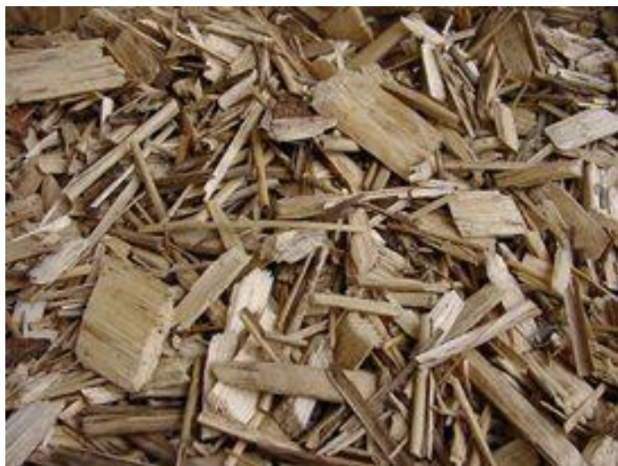
Figure 5.12 Wood chips and reed mixture (20% reed by volume) (Photo: Ü. Kask)
