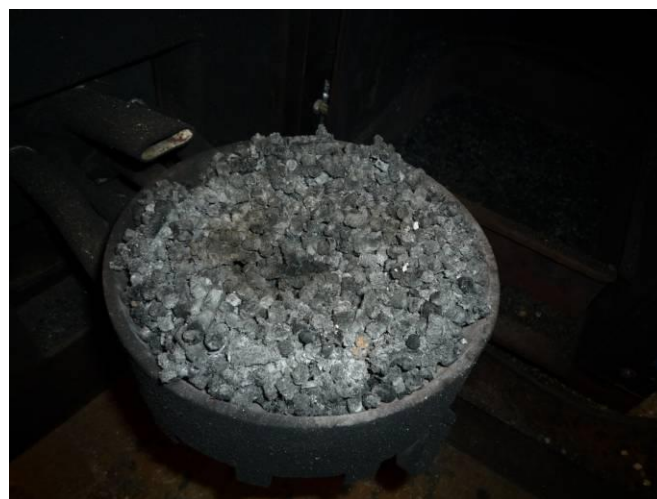
Figure 4.14 Combustion residues after test (Photo: Ü. Kask)
