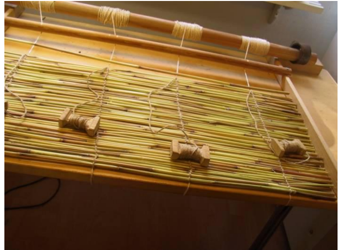
Figure 7.6 Simple version of a rug loom makes it easy to weave a reed rug or a seat cushion (Photo: O. Tuomela)
