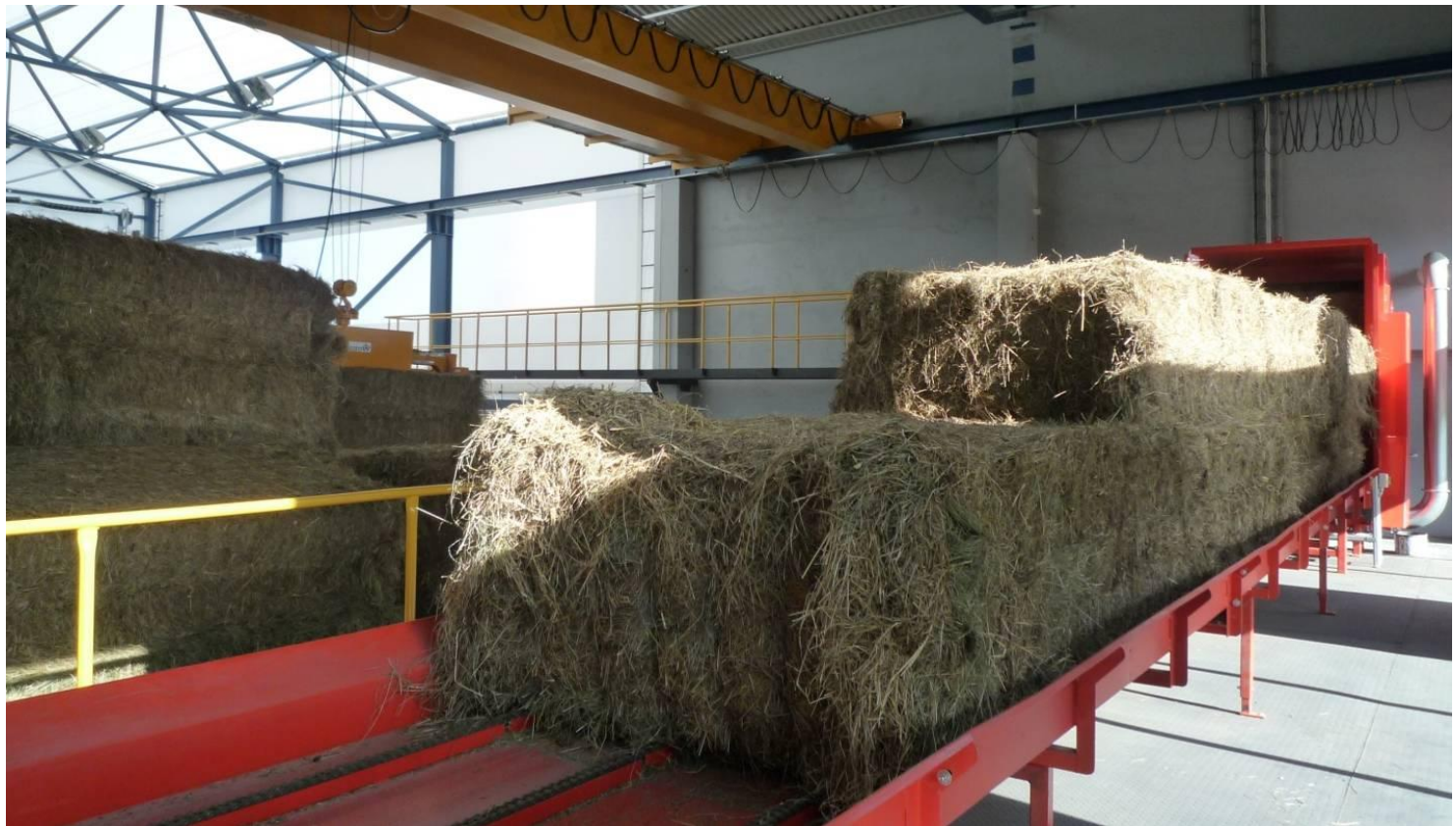
Figure 4.8 Hay (left) and reed on a conveyer belt at Lihula Boiler House (Photo: Ü. Kask)
