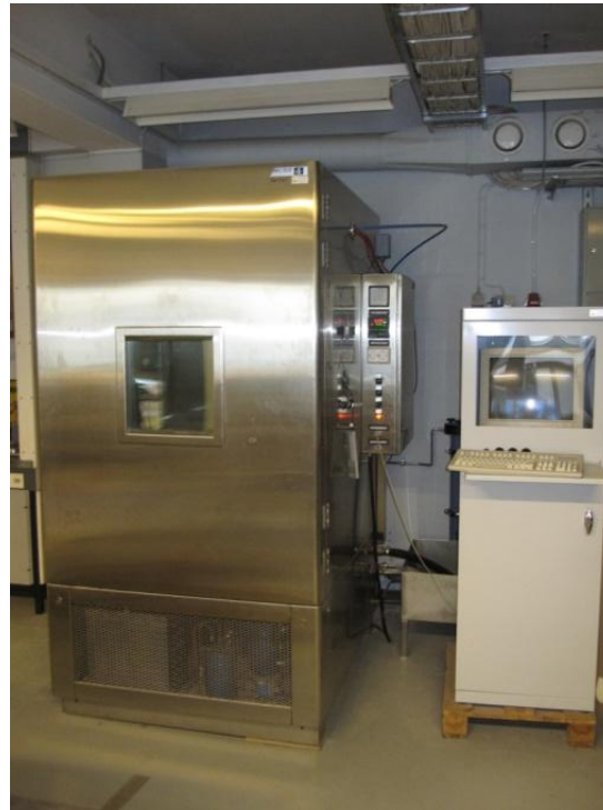
Figure 3.28 ARCTEST 1500 climatic test chamber
