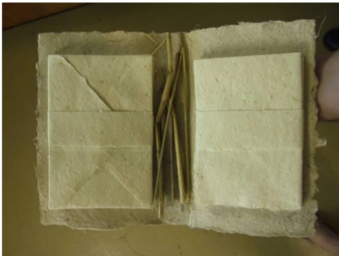
Figure 7.8 Reed harvested in summer has the highest fibre content and it can be used for making light brown paper (made by Biopap Oy Fiskars) ( Photo: O. Tuomela)
