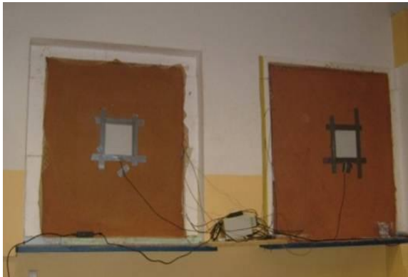
Figure 3.14 Heat flow plates to measure the heat transmittance and thermocouples to measure the temperature of surfaces of the wall fragments
