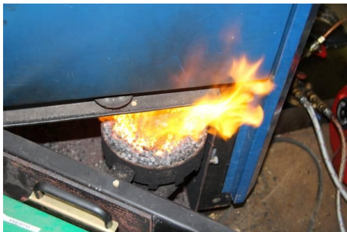
Figure 4.13 Pellet burner BioLine 25 (Sweden) (Photo: Ü. Kask)
