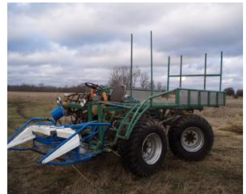
Figure 3.4 Self-made reed harvesters belonging to Thatched Roof OÜ (Photos: Reedroof 2010)
