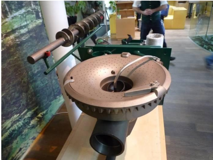
Figure 4.10 The ring nozzle burner (Photo: Ü. Kask)
