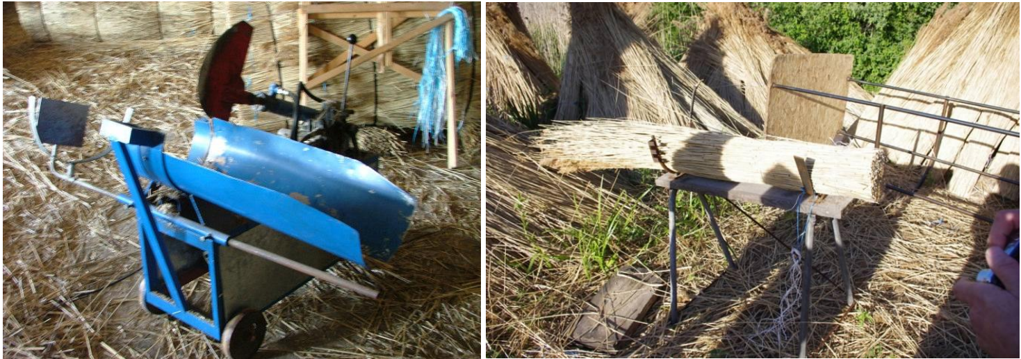
Figure 3.5 Reed bundle binding bench, on the left in Estonia, on the right in Latvia (Photos: J. Miljan)
