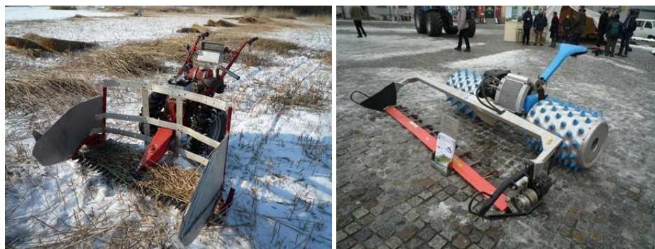
Figure 5.3 Small engine-driven BCS mower (left), mower with a wide heeder (right)
