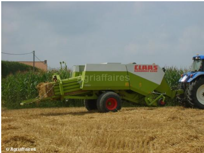
Joonis 5.7. Suur heinapakipress Claas ( http://classified.fwi.co.uk/browse/grassland-equipment/balers/big-square-balers )
