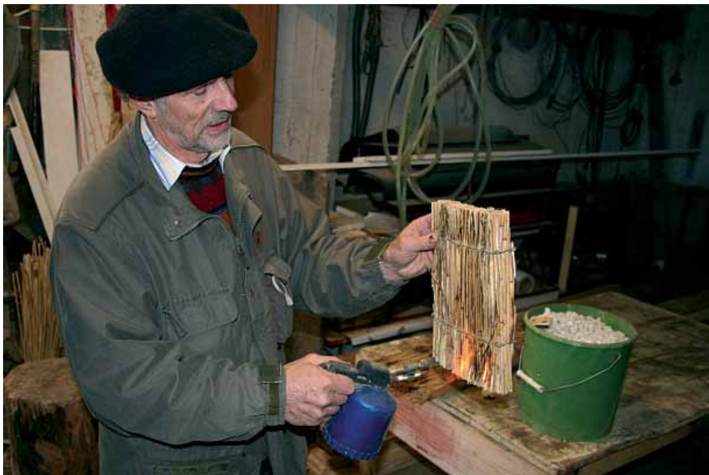
Hartwig Reuter is “trying” to burn part of a Berger plate, which is an insulation plate made of reed. This thick plate is not easy to burn. Photo: Iiro Ikonen.
