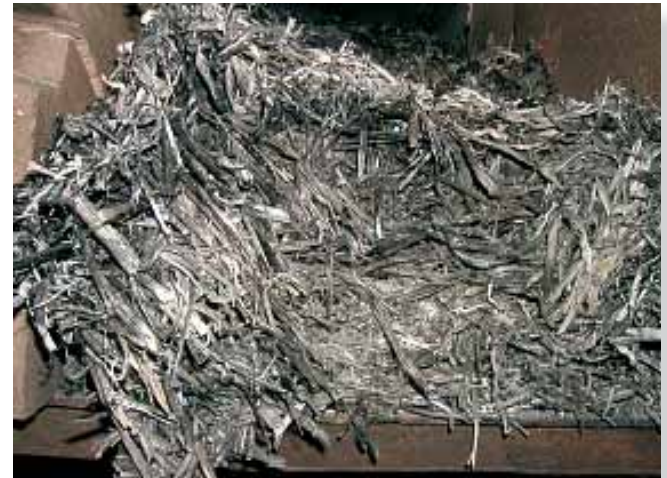
Reed ash residue after combustion. Photo: Ülo Kask.
