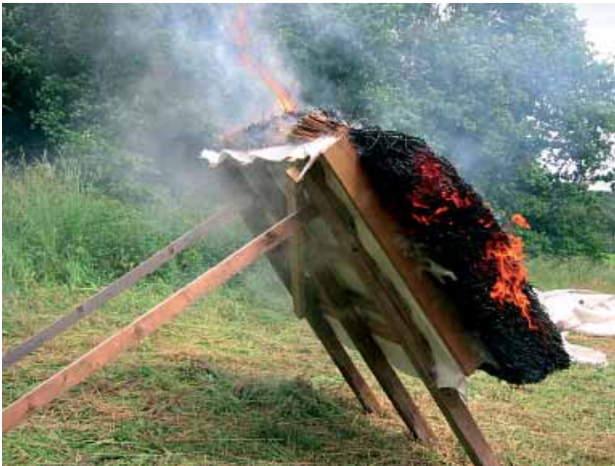
A burning test with a small reed-roof model. Photo: Carlo F. Christensen.
