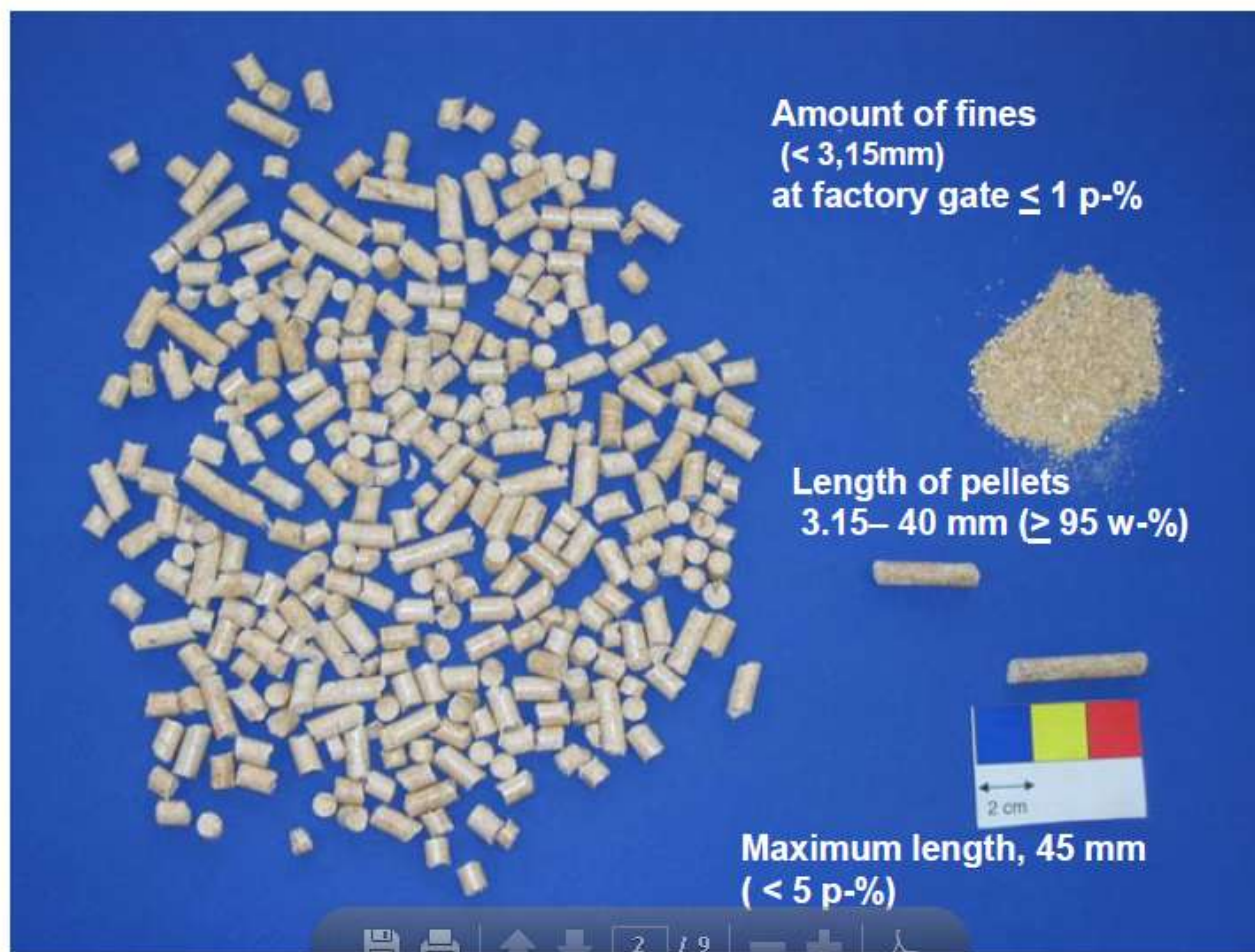
Fig 2. Dimensions of 8 mm wood pellets according to EN 14961-1.
