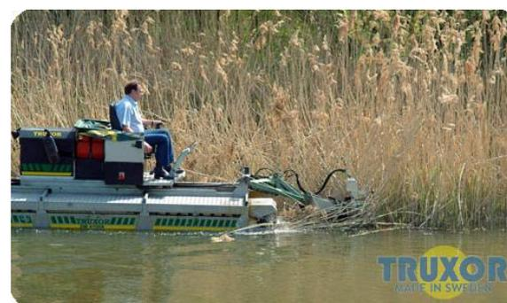
**Figure 5.5.** Floating mower Truxor Doroklippen ESM 2100 (<http://doroteamekaniska.se/2esm2100.html>)
