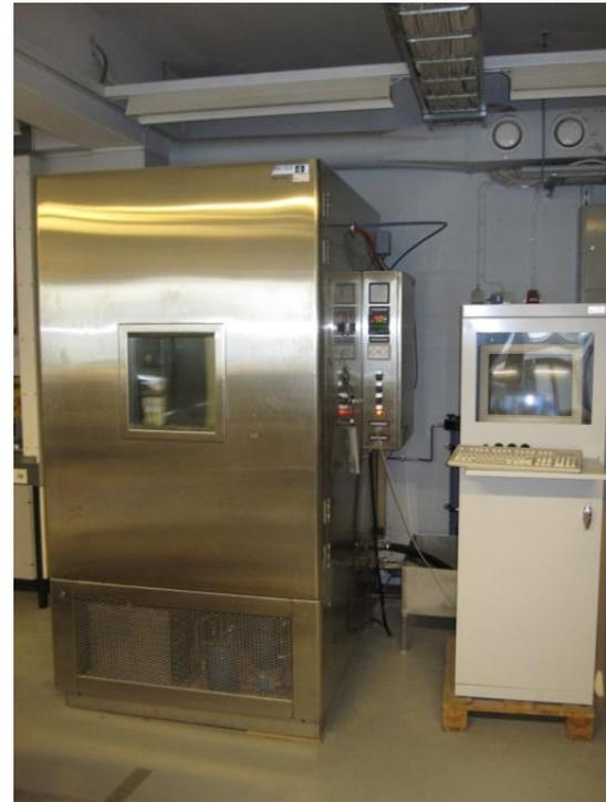
**Figure 3.28.** ARCTEST 1500 climatic test chamber
