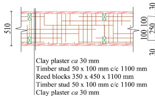
**Figure 3.20.** Different wall structures of test house
