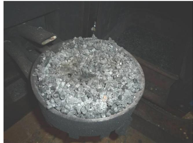
**Figure 4.14.** Combustion residues after test (Photo: Ü. Kask)
