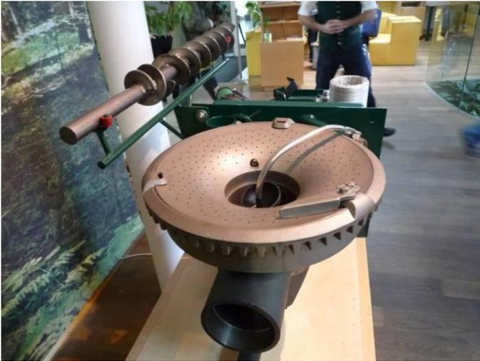
**Figure 4.10.** The ring nozzle burner (Photo: Ü. Kask)
