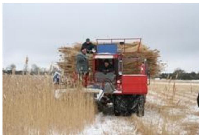
**Figure 5.8.** Reed cutter Seiga BCS (Photo: Ü. Kask)
