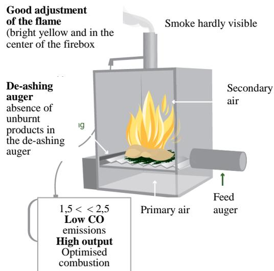
**Figure 4.15.** Layout of the test boiler
