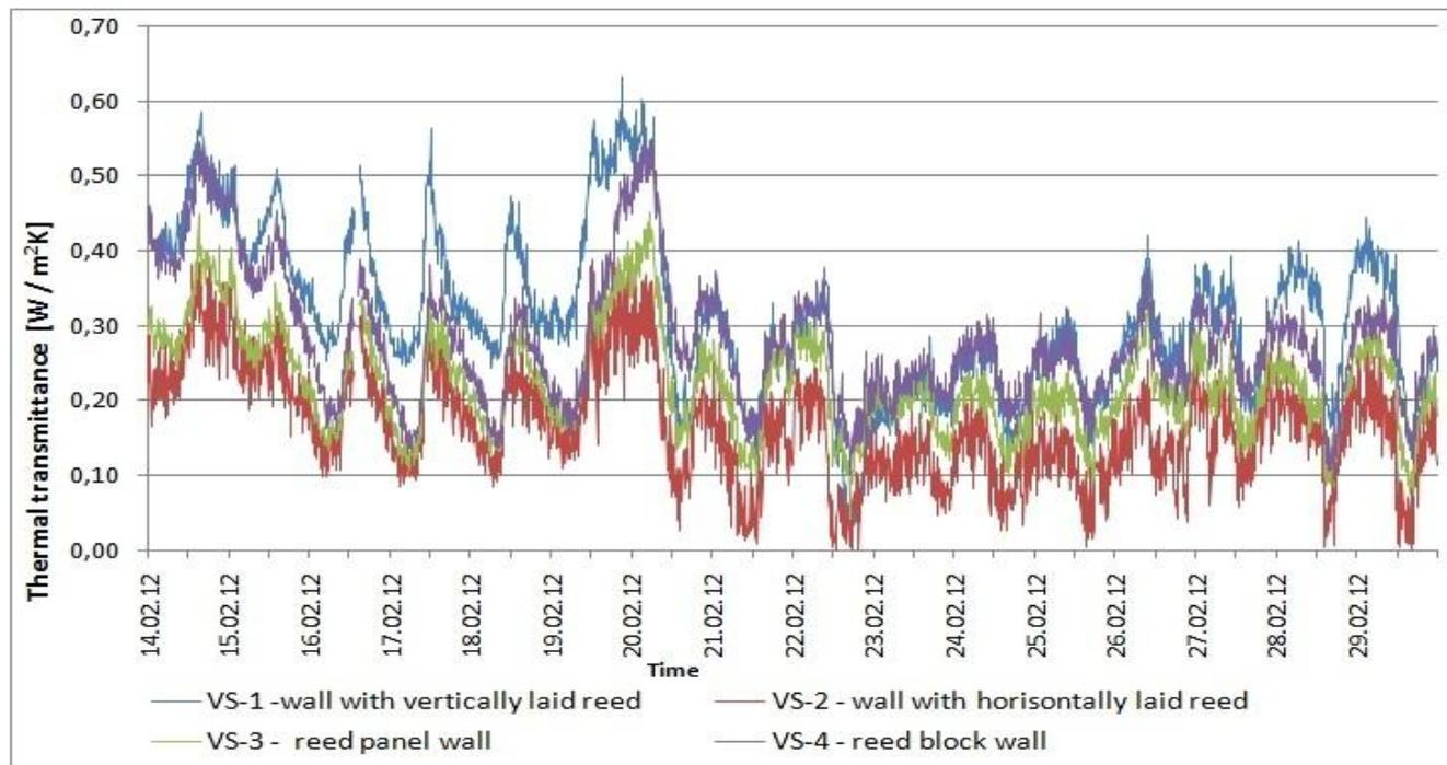
**Figure 3.25.** Changes in thermal transmittance of different test walls in non-steady environment (2<sup>nd</sup> half of February 2012) (Miljan M-J. 2012 c)
