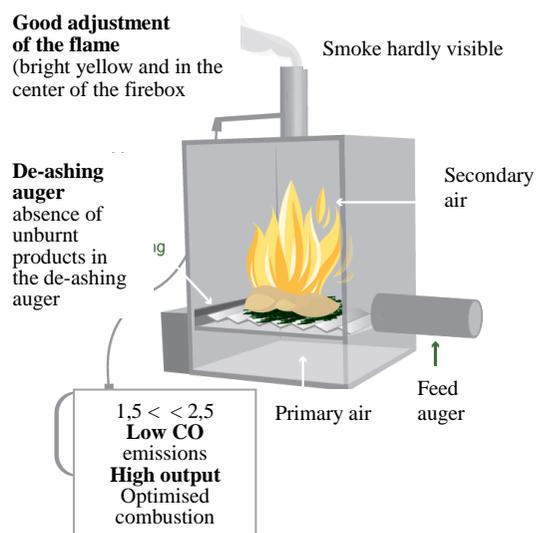
**Figure 4.15.** Layout of the test boiler
