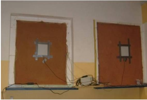
**Figure 3.14.** Heat flow plates to measure the heat transmittance and thermocouples to measure the air-temperature inside and outside
