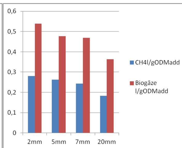
**Figure 6.2.** Average biogas and methane output from green reed, different cut sizes, l/g<sub>ODM</sub>
