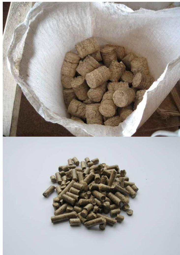
**Figure 4.4.** Reed pellets (lower) and reed briquettes (upper) (Photo: Ülo Kask)
